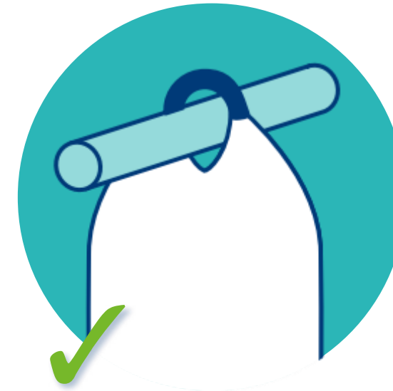
Only lift Big Bags by the specially designed lifting strap and lifting equipment with rounded corners.
