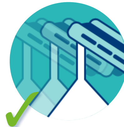
Move the discharge point regularly while filling the bulk storage bin, to avoid segregation.
